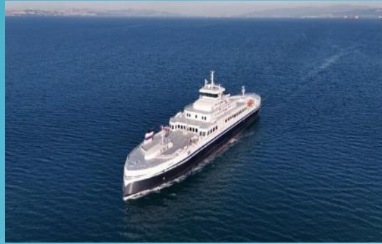
CEMRE SHIPYARD Ferry/Ropax Largest Zero Emission Freight Ferry Diesel/ Battery (10 MWh battery) Upgrade to Methanol
