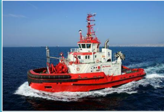
SANMAR SHIPYARD The World's 1st LNG Fuelled Escort Tug
