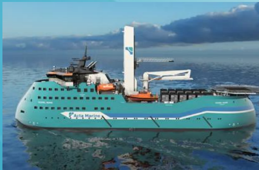
TERSAN SHIPYARD Construction Service Operating Vessel (CSOV) Methanol-Marine Diesel Oil (MDO)/HVO Powered DP2
