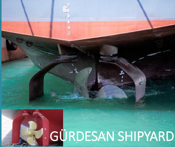
Erge: First Gate rudder Retrofit (2023)
