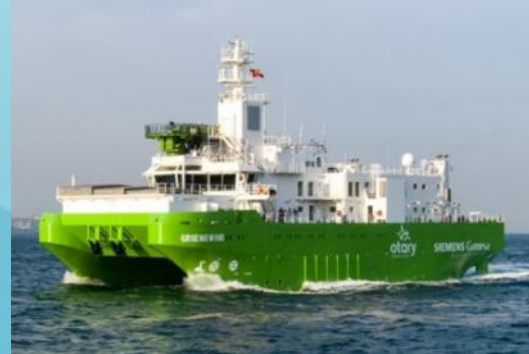
CEMRE SHIPYARD The World's 1st DP2 SWATH Type Service Operation Vessel Powered by Batteries and Dual Fuel /Methanol
